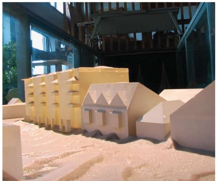
Snow accumulation study using silica sand in the water flume
