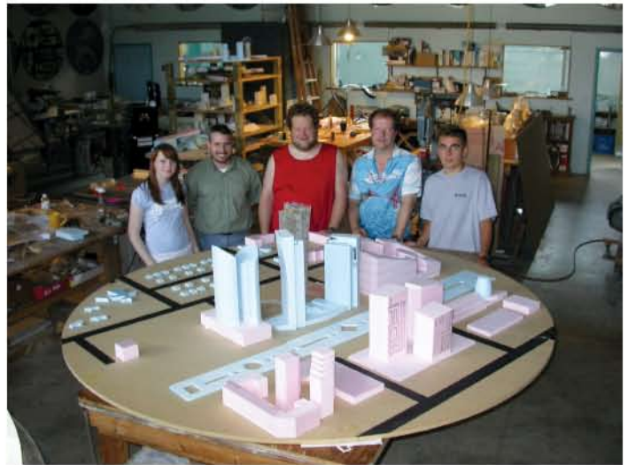
Wind Tunnel model used to assess wind pressure on cladding and structural loading
